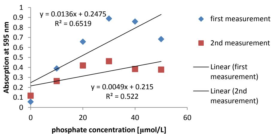
**Problems:** Our calibration curve cannot be fitted by a straight line. During the first measurement too many mistakes were made, the results could not be used.
