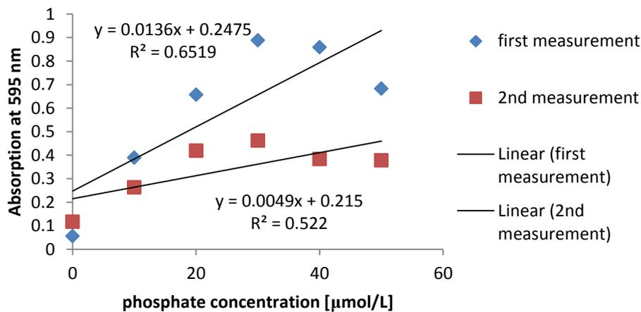
**Problems:** Our calibration curve cannot be fitted by a straight line. During the first measurement too many mistakes were made, the results could not be used. However, it would be quite ok for the first 4 values. In our second measurement we got a straight line for the first four values, the last two values lay unfortunately not on the straight line.
